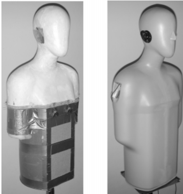
Figure 8: Figure 8: Left: The final prototype made in wood and plaster. Right: A new model made in plastic.
