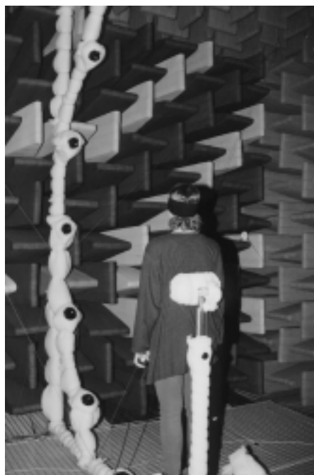
Figure 2: The HTTF measurement setup in the anechoic room.
